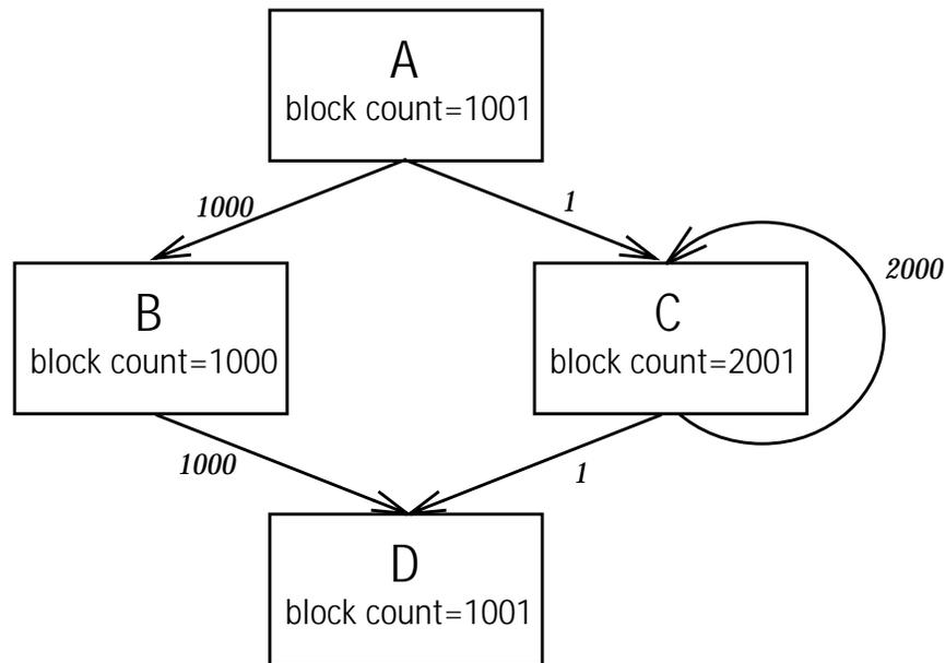
**Figure 7.2 An Example Where Edge Counts Can Be Derived From Block Counts.** An unknown count for an edge  $(X, Y)$  can be calculated if it is the only unknown successor of block  $X$ , or the only unknown predecessor of block  $Y$ . Repeated application of this rule until convergence can often calculate all edge counts, as in this example. (An augmented version of Figure 3 from [69].)
