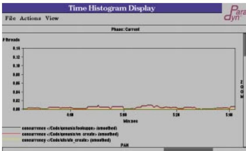
**Figure 6.12 `vn_create` Time With Both the File Truncation and DNLC Optimizations Applied.** *`vn_create` once consumed 40% of Squid's run time (Figure 6.4); that number is now less than 1%.*
