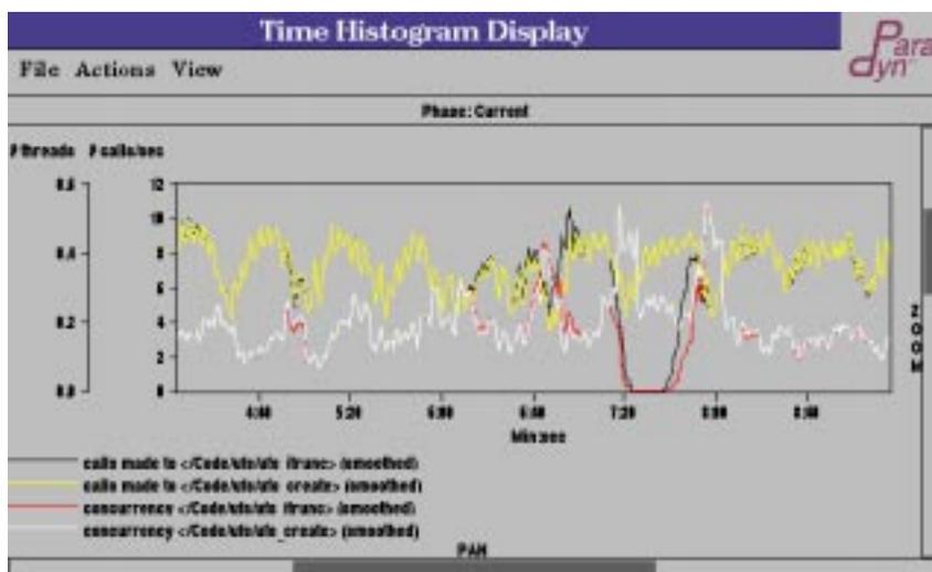
**Figure 6.5** `ufs_create` Time is Spent Primarily in `ufs_itrunc`. *UFS file creation time is dominated by inode truncation; the concurrency curves for `ufs_create` and `ufs_itrunc` almost completely overlap.*
