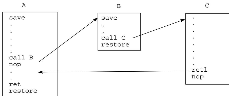
**Figure 3.3 Tail Call.** *In this example, function B (called from A) makes a tail call to C. B has a restore instruction in the delay slot of the call to C, which changes to A's stack frame. The link register now contains the address in A where it calls B, so C will return directly to A.*
