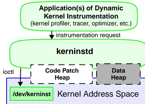
**Figure 3.1 KernInst System Architecture.** *Kerninstd acts as an instrumentation server, performing kernel instrumentation requests that arrive from applications.*
