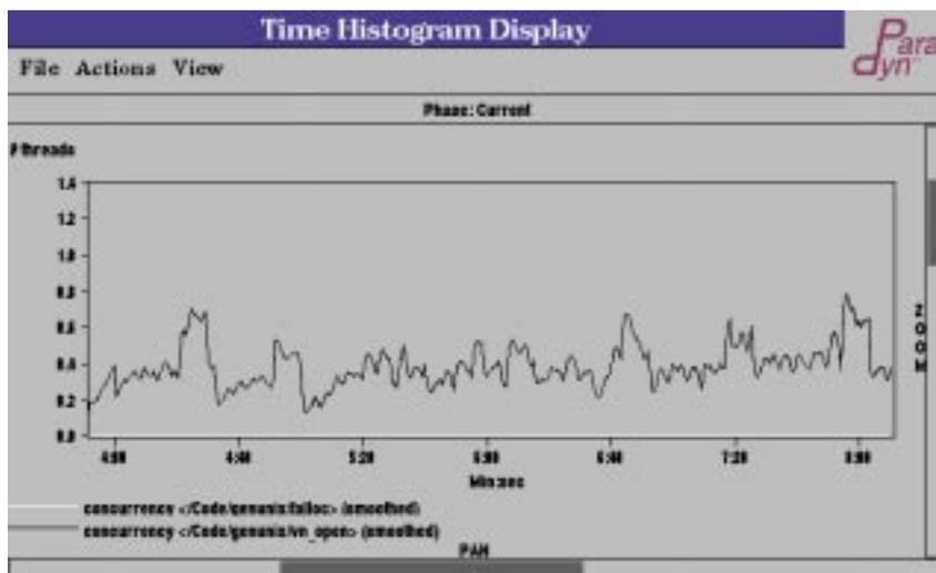
**Figure 6.2** The Major Callees of `copen`: `falloc` and `vn_open`. `vn_open` accounts for almost all of the time spent in `copen`; negligible time is spent in `falloc`.
