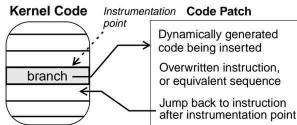
**Figure 4.1 Code Splicing.** One machine code instruction is overwritten with a branch to patch code, which contains the desired instrumentation code, the overwritten instruction, and a branch back to the instruction stream.
