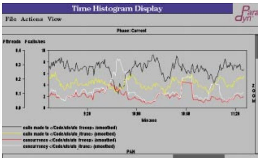
**Figure 6.11 ufs\_itrunc in Optimized Squid.** *Because Squid no longer uses the O\_TRUNC flag opening cache files, truncation is now mostly performed when explicitly requested via fcntl (ufs\_freesp).*
