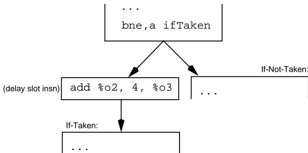
**Figure 3.2 Conventional Placement of Conditionally Annulled Delay Instruction.** *The delay slot instruction (add %o2, 4, %o3) is placed in its own basic block, reachable only when the branch is taken. Unfortunately, this single-instruction basic block is not an efficient use of memory for KernInst’s control flow graph or live register analysis.*
