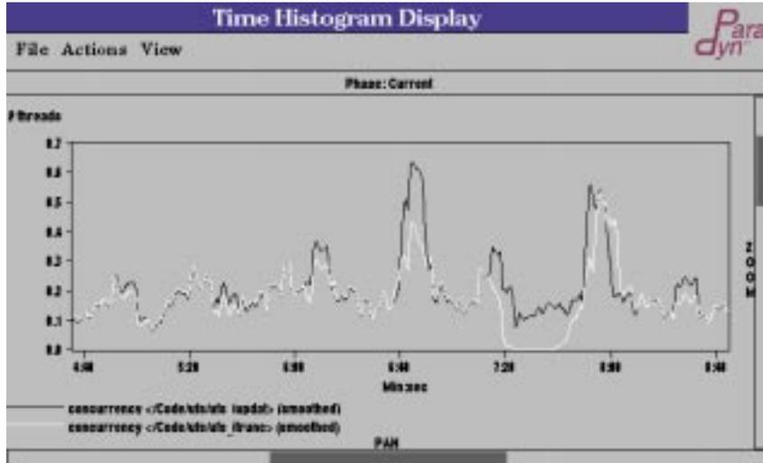
**Figure 6.6** Most of `ufs_itrunc`'s Time is Spent in `ufs_iupdat`. File truncation is slow because UFS meta-data updates are made synchronous by `ufs_itrunc`.
