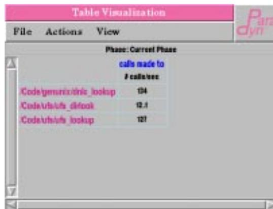
**Figure 6.7** The DNLC Hit Rate. The miss routine, `ufs_dirlook`, is only invoked once per 10 calls to `ufs_lookup`, for a DNLC hit rate of about 90%.
