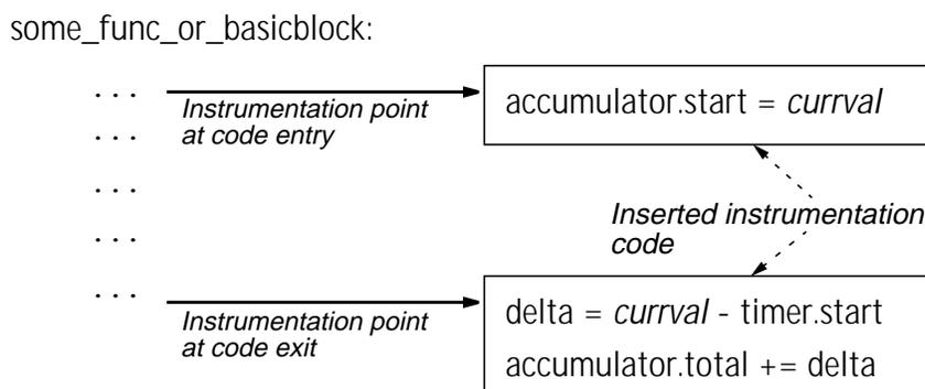
**Figure 1.1 Interval Counter Accumulation Instrumentation.** *Currval is the current value of the metric's underlying event counter, such as elapsed cycles or number of cache misses. This diagram omits several details, such as making the instrumentation code thread-safe, that will be discussed in Chapter 5.*
