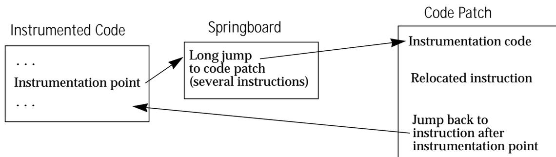
**Figure 4.7 Using Springboards to Reach the Code Patch.** *A level of indirection is used to reach the code patch from the instrumentation point. When finished, the code patch returns directly to the instrumentation point.*
