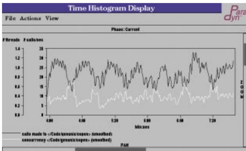
**Figure 6.1** `copen`. Although called only 20-25 times/sec, `copen` is a clear bottleneck. On average, 0.4 kernel threads are executing in this routine at any given time. This number translates to 40% of Squid's elapsed time, since Squid is a single-threaded program.
