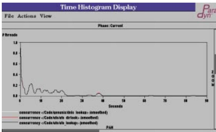
**Figure 6.9 The Effect of Increasing DNLC Size on ufs\_lookup Latency.** *For the first twenty seconds of the benchmark, there are enough DNLC misses to account for 10% of Squid's run time. As file names are reused more often, however, the DNLC hits become more frequent, and the ufs\_dirlook bottleneck evaporates (compare to Figure 6.8).*
