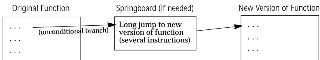
**Figure 4.9 Basic Code Replacement.** *The entry point instruction of the original function is replaced with an unconditional non-delayed branch to the new version of the function. A springboard is used if needed.*
