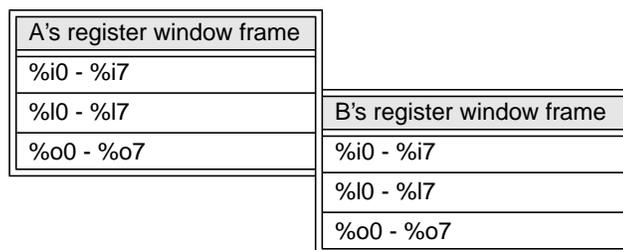
**Figure 3.6 SPARC register window overlapping.** *In this example, A has its own register window frame. It then calls B, which sets up its own frame by executing a save instruction. B gets a new set of %l and %o registers, and its %i registers overlap with (i.e., are aliases for) the previous frame's %o registers.*
