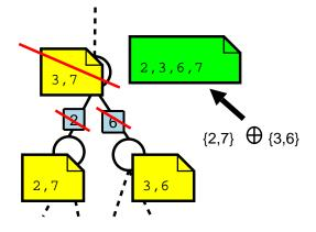
Figure 2: To compensate for the lost filter and channel state after failure of the subtree's root, computationally consistent state obtained by composing the failed process' children's states is used.
