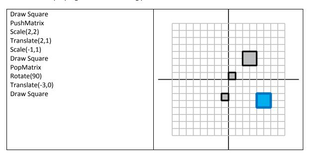
**A:** If we forgot the "Push Matrix" and "PopMatrix" commands in the example program, the last square would appear in a different place. Draw it on the example above.
